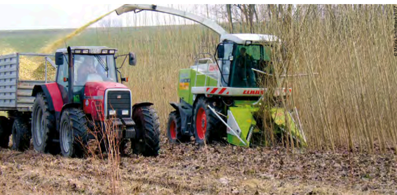
Poplar harvest in short-rotation forestry: after three years of undisturbed growth, the tree trunks are cut down and shredded.
