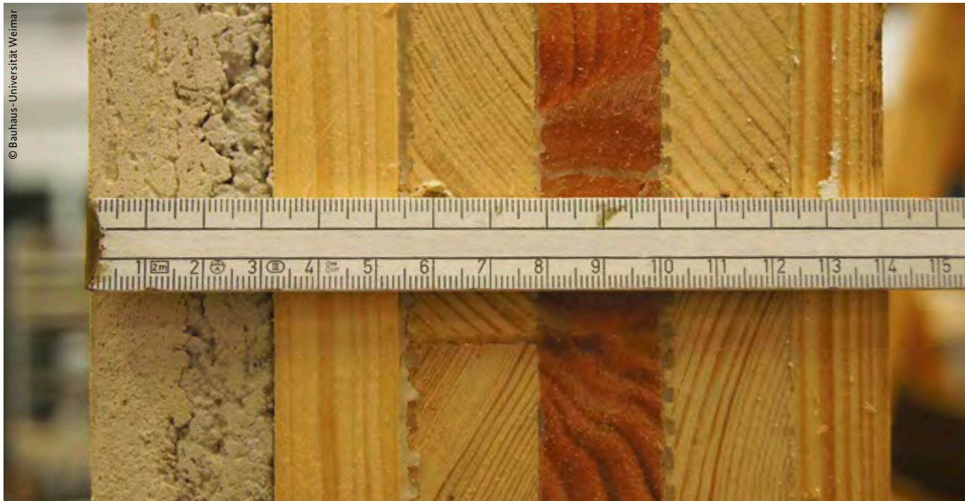
Able to support great loads, and good for indoor climate: in wood-anhydrite composite systems, civil engineers from Bauhaus University in Weimar apply anhydrite, similar to gypsum, directly onto wood.
