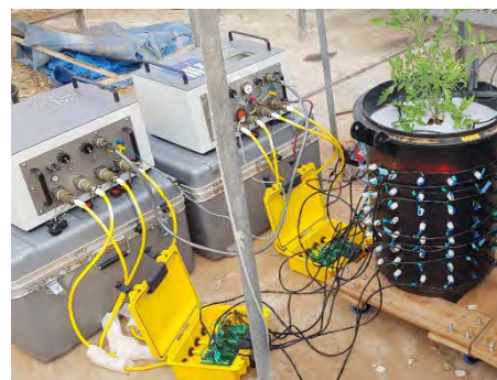
Figure 2: The lysimeter system during an electrical survey.
