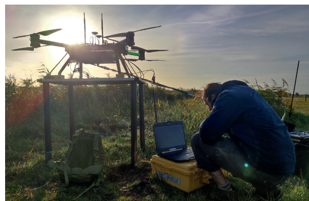
The SeeKaquA project uses a new drone-based measuring system to detect aquifers.
